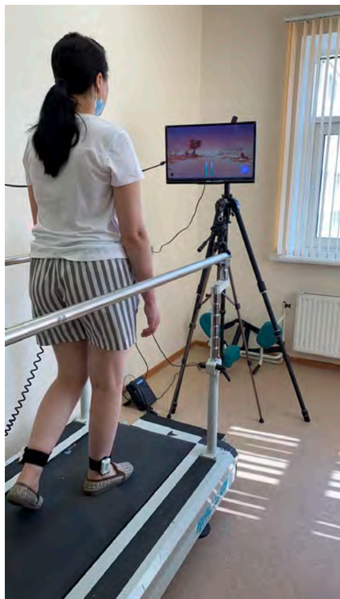
Training process. The patient is on a treadmill. Inertial sensors are installed on his shins to register gait parameters. Before him is a screen with a virtual task.
